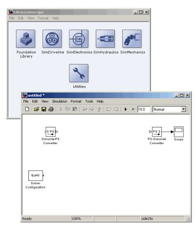
By default, the model name is not specified, the model contains a Solver Configuration block with the default solver set to ode15s, a Simulink-PS Converter block, and a PS-Simulink Converter block connected to a Scope block.
